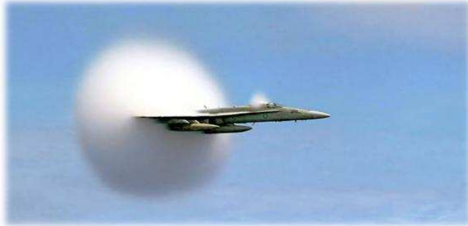
Figure 1.5: Snapshot of shock condensation effect around the jet fighter Boeing F-18 (Hornet) at transonic flight in humid air. It arises during acceleration when the air flow at some parts of the fuselage reaches supersonic speeds. When the resulting shock wave detaches, it builds up a sudden rarefaction that, lowering the temperature, causes condensation of the ambient water vapor.[Courtesy: J. GAY, U.S. Navy] A similar picture was recently taken from an F-4 (Phantom II) during an air show at Point Magu Naval Air Station, CA. (The MilitaryAircraft Archive, http://www.milair.simplenet.com/ )
