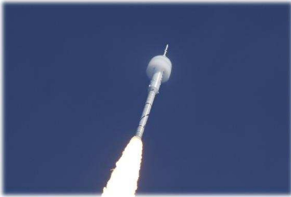
Figure 1.6: Snapshot of the bow shock wave formed due to the supersonic flight of the NASA's new Ares -1X rocket
